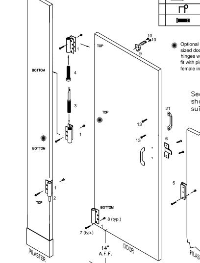
Optional third hinge may be used for larger sized doors. Mount between two standard hinges with pilaster side hinge as lower half fit with pin. Door side will be upper and fit female insert.
