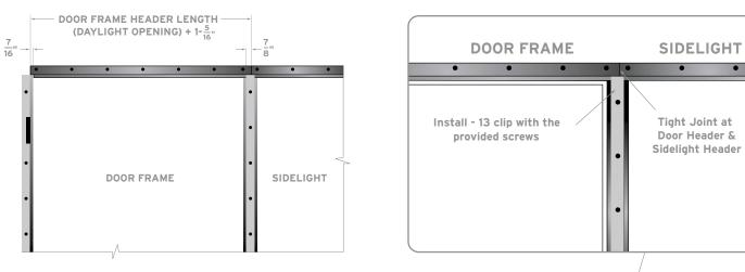
5th. STEP: INSTALL THE SIDELIGHT MULLION USING ALUMINUM CLIP NOTE: SIDELIGHT MULLION BUTTS UP TO HEADER SEE ATTACHED DETAIL
