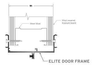
V. Moving over to the partition side of the sidelight, cut the sidelight glazing post for the partition side of the sidelight. Do this by measuring from the underside of the header to the floor or rough sill. Cut and install this jamb, plumb using 2 screws. Insure the header bypasses the jamb by  $\frac{71}{16}$ . See "figure [b]"
