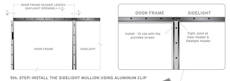
5th. STEP: INSTALL THE SIDELIGHT MULLION USING ALUMINUM CLIF NOTE: SIDELIGHT MULLION BUTTS UP TO HEADER SEE ATTACHED DETAIL
