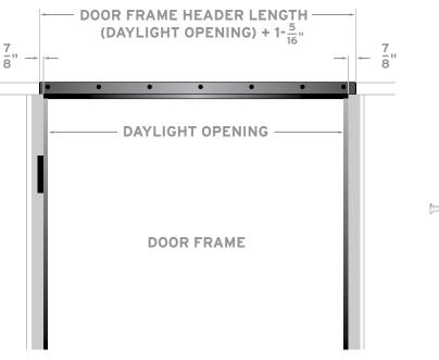
IV. Continuing to work on the same side of the opening, locate, level and fasten the sidelight header. This header should be cut to its correct size as well, depending on the size of the sidelight width required. Once again, this is the desired daylight opening width plus  $1 \frac{5''}{16}$ .
