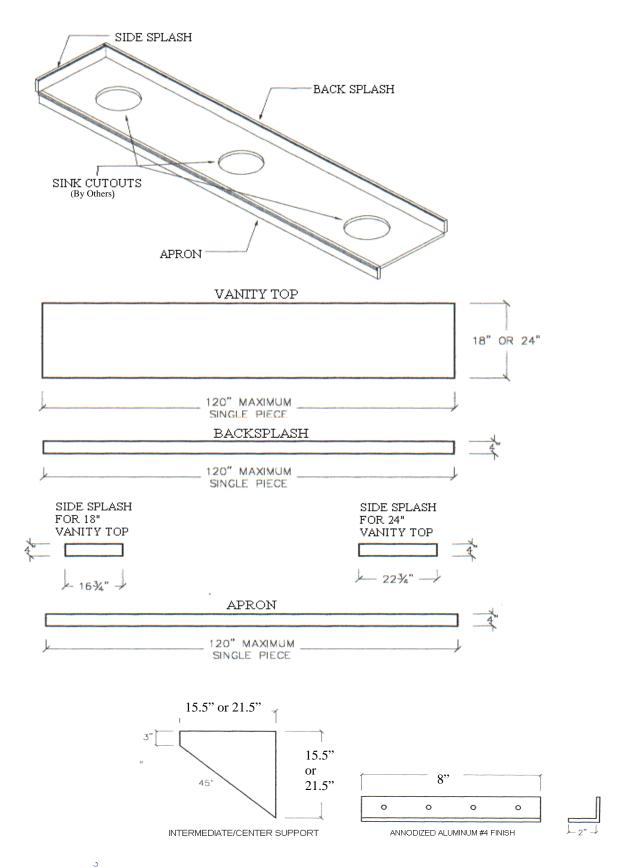
END SUPPORT AND INTERMEDIATE/CENTER SUPPORT ARE BOTH 1" THICK HDPE. INTERMEDIATE/END SUPPORT SHALL BE EVENLY SPACED AT A MAXIMUM OF 36".
